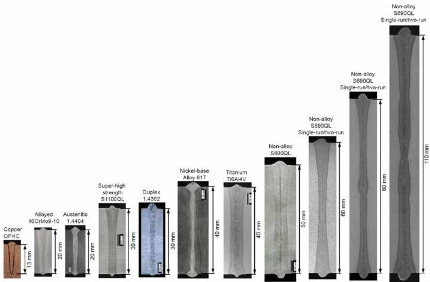
Potential weld cross-sections and weldable materials when being used in a laser beam welding process and placed under a vacuum.
